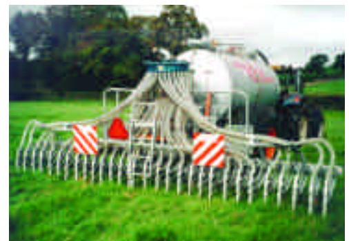
Trailing shoe band spread slurry application.
